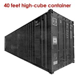
The 40 feet high cube container it is similar to the standard 40' with and extra feet tall. The standard one has 8.5' and the high cube has 9.5' tall, this means a 13% of it's inner capacity.
