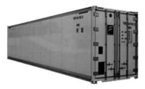
New. The last generation of high cube containers, developed to frozen cargo or refrigerated, recommended to transport perishable items like food, with a range from -30° to +50°.
