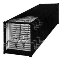
The 20' ventilated container was designed to an specific type of cargo, the ones that must have a constant temperature, because of it's amount of humidity. It has two fans at each side, the roof and floor working all around the container. The warm air flows through the roof vents while the cool air goes in through the vents on the floor.
