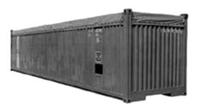
It was developed to move certain items that can't fit through doors. Without roof, the cargo goes in through the top of the container. A canvas goes through the hooks and covers and protects the cargo. The container has an open roof built in 20 and 40 feet tall.
